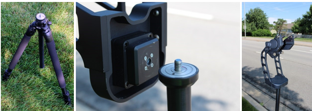
Figure 2-59 – Tripod base, yoke & tripod post, assembled yoke on tripod
