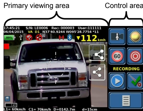
Figure 2-2 - Enforcement Screen on Rear Display
