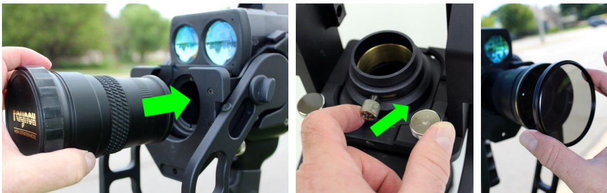
Figure 2-61 – Zoom Lens Mount, Lens Lock, Polarizing UV Filter
