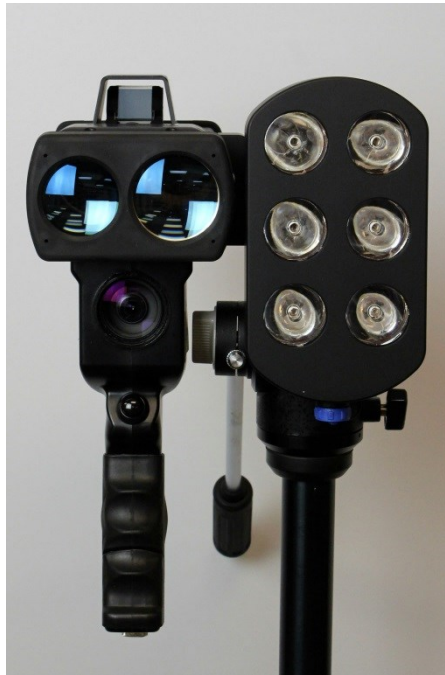
Figure 1-9 – LaserCam 4 with IR Illuminator
